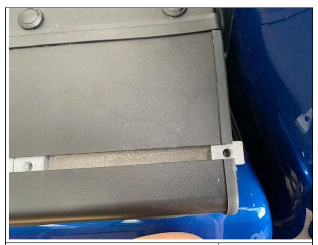
20. Fit 6x small rectangular nuts into slot on roller shutter per side.
