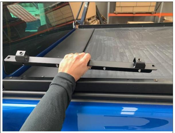
23. Drop Tub Rail assy on top roller shutter mount and secure with at least 4 M8 screws per side.
