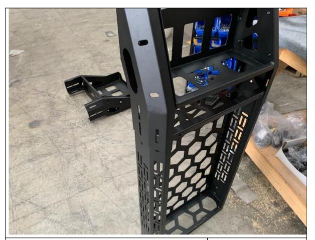
5. Slide side arm assembly over centre basket as shown and loosely fit M8 hardware to keep arm attached. Leave all hardware loose.
