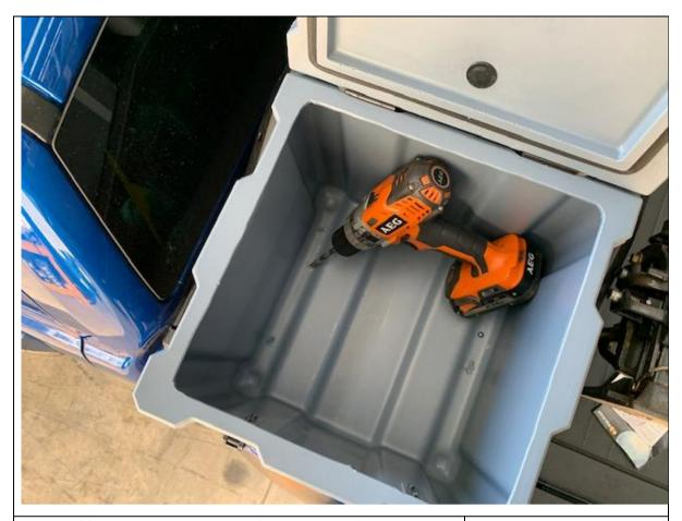
29. If fitting small space case to flat basket, you'll need to drill holes in from inside box and secure down. This will allow you to open the box without removing it, and prevent it from being stolen.
