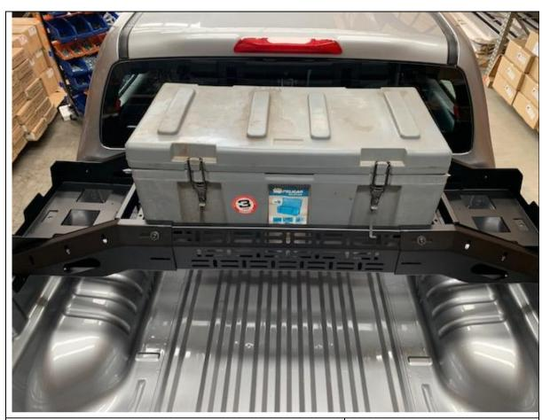
32. If fitting centre space case, secure down with ratchet strap running from handle to handle underneath rack so you can still open the box.
